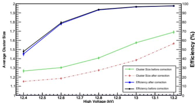
More than 95% efficiency is achieved at the operating voltage of 13.0 kV while the cluster size remains less than 1.4 after applying the corrections. No visible reduction in the efficiency has been observed after correction, whereas the cluster size reduces after correction
