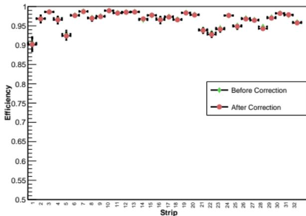
RPC plateau efficiency distribution at 13 kV for all the strips. No significant reduction in efficiency has been observed after neglecting the events which show noisy events or multiple cluster hit in the detector within fixed interval.
