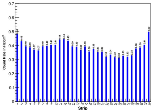
The count rate is determined independently for each strips by counting the number of hits that are above the discrimination threshold per unit area of the strip.
