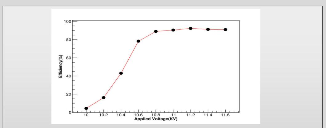
Working Point: the lower the better (Electric field play a key role: The impurities in the gas, which are transported with the gas flow may directly deposit on the surface of electrodes due to electrostatic forces)
