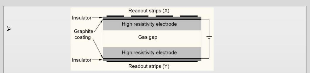
The Resistive Plate Chamber (RPC) was developed in 1981 by R. Santonico and R. Cardarelli.
