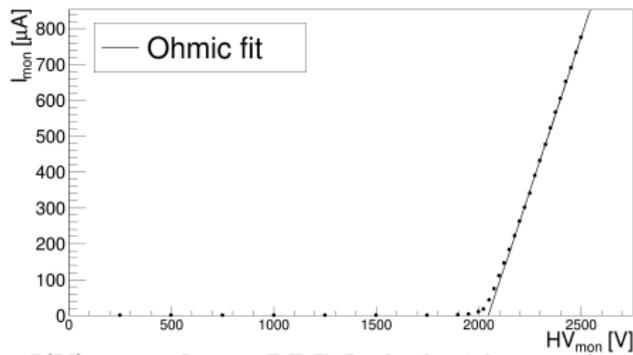
$I(V)$  curve for an RPC flushed with pure Ar
