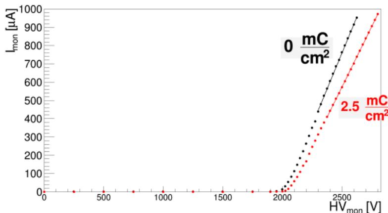
Different I(V) curves in Ar for different values of integrated charge
