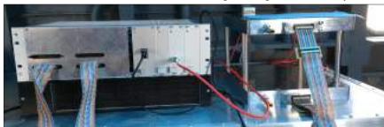
Detectors assembled with readout and high voltage electronics system
