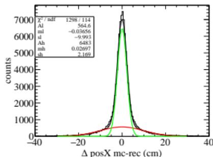
The resolution leak in cosmic rays detection is due to low energy muons interaction with medium. This effect does not depend on intrinsic detector resolution (see **2018 JINST 13 P08026**).
