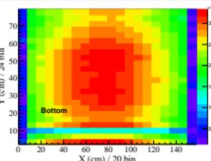
Hit distribution for each chamber of TORI-03 telescope.
