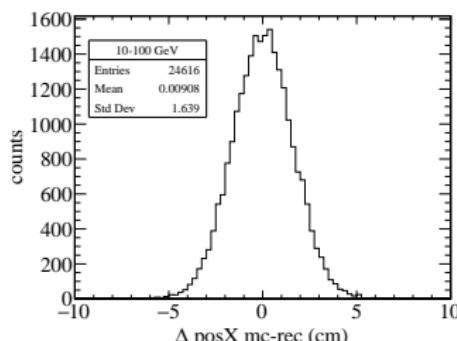
Differences between the generated and reconstructed polar angle, X and Y positions in middle chamber. High energy muons make the effects due to air medium negligible, then we use them to estimate the detector resolution.
