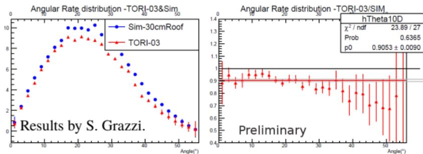
Red triangles represent the polar angle distribution of data collected by TORI-3, while the blue circles are the same distribution obtained by simulating a sample with the same statistic but without detector efficiency information
