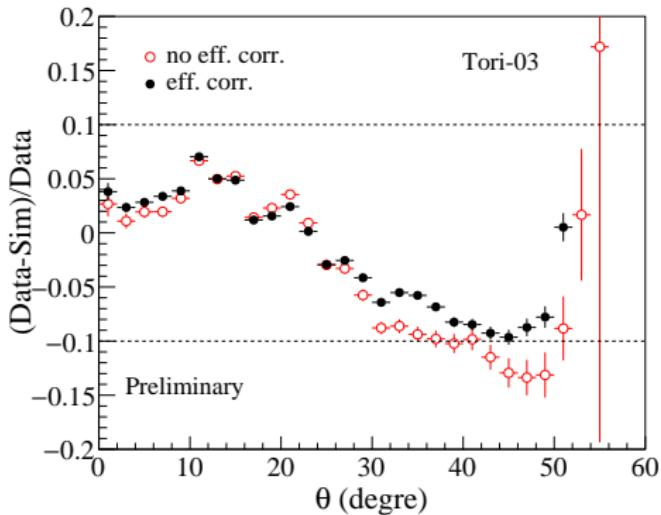
The experimental and simulated polar angle data, without correction (open circles) and with the efficiency correction (full circles) are in agreement within 5-6% in both cases for polar angle below 35 degrees, with efficiency correction the agreement remains within 10% above 35 degrees.
