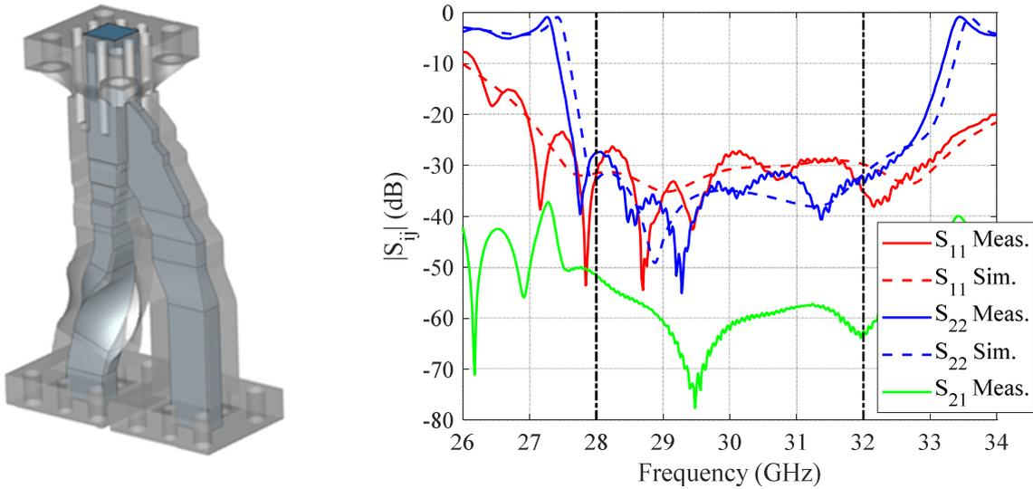
Fig. 3. Ka-band orthomode transducer integrated with a 90-deg twist. Left: 3D CAD of the component optimized for selective laser melting manufacturing. Right: comparison between measured and predicted performance of the prototype.
