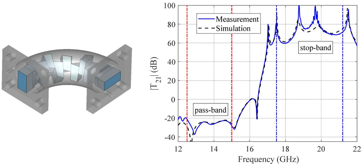
Fig. 2. Ka-band orthomode transducer integrated with a 90-deg twist. Left: 3D CAD of the component optimized for selective laser melting manufacturing. Right: comparison between measured and predicted performance of the prototype.
