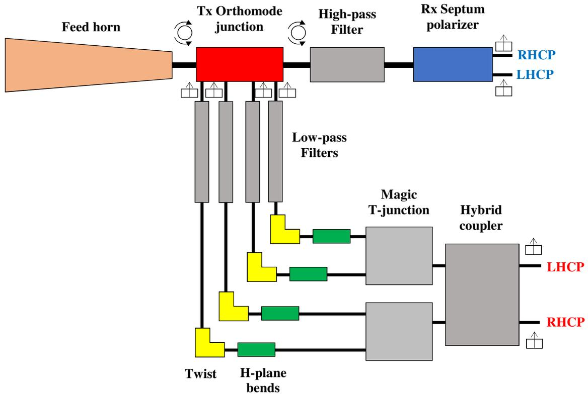
Fig. 1. Block diagram of a dual-band dual-polarization antenna-feed chain for multi-beam Space applications.
