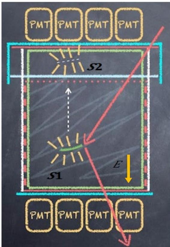
The basic idea of Columnar Recombination: for nuclear recoil parallel to the electric field, more electron-ion recombination is expected since the electrons must traverse more ionized medium as they drift.
