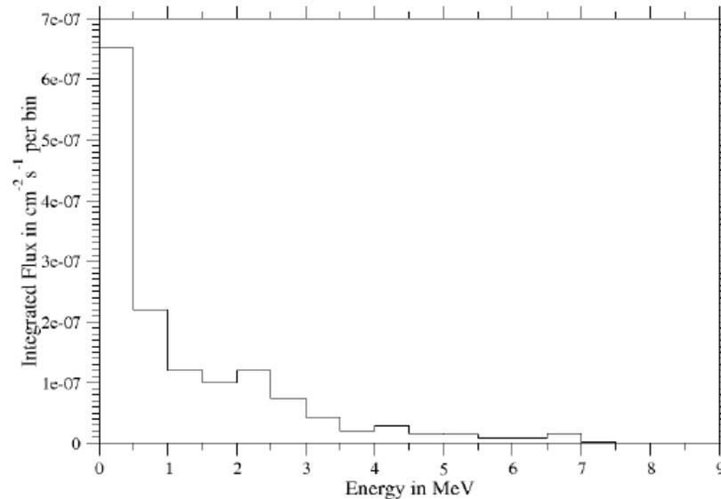
Integrated Flux above 500 keV:  $\sim 7.9 \cdot 10^{-7} \text{ n cm}^{-2} \text{ s}^{-1}$
