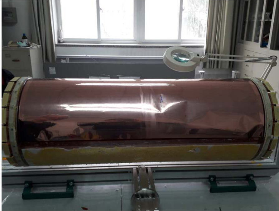
Figure 2 – The Layer 3 opened. The damage to the GEM foil is visible.
