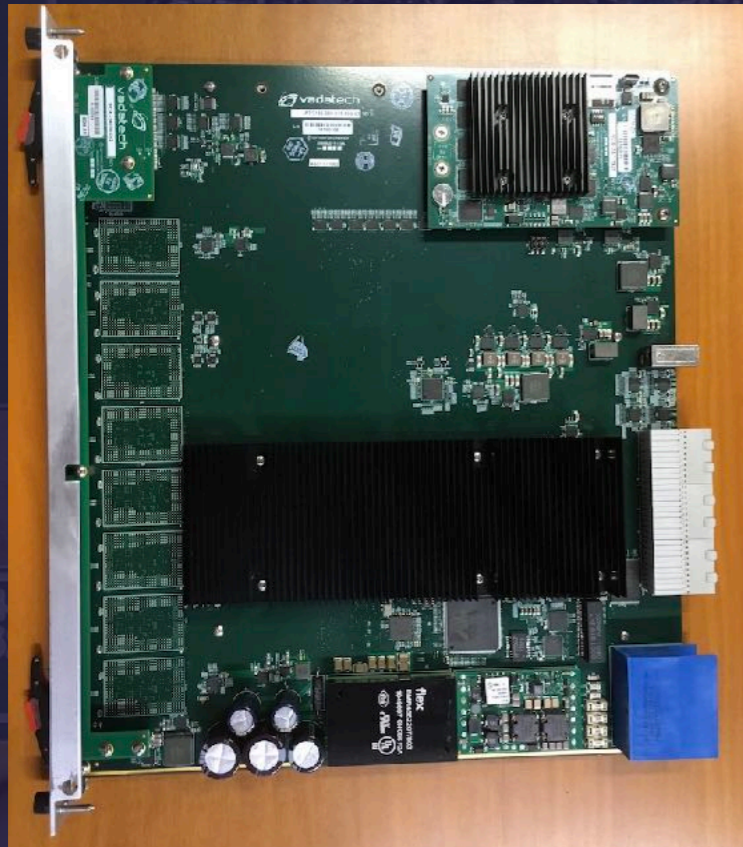
ATCA blade 35 x 28.5 cm 2 Vadatech ATC136 modified Xilinx Virtex-7 FPGA Four core QorIQ P2040 Power PC
