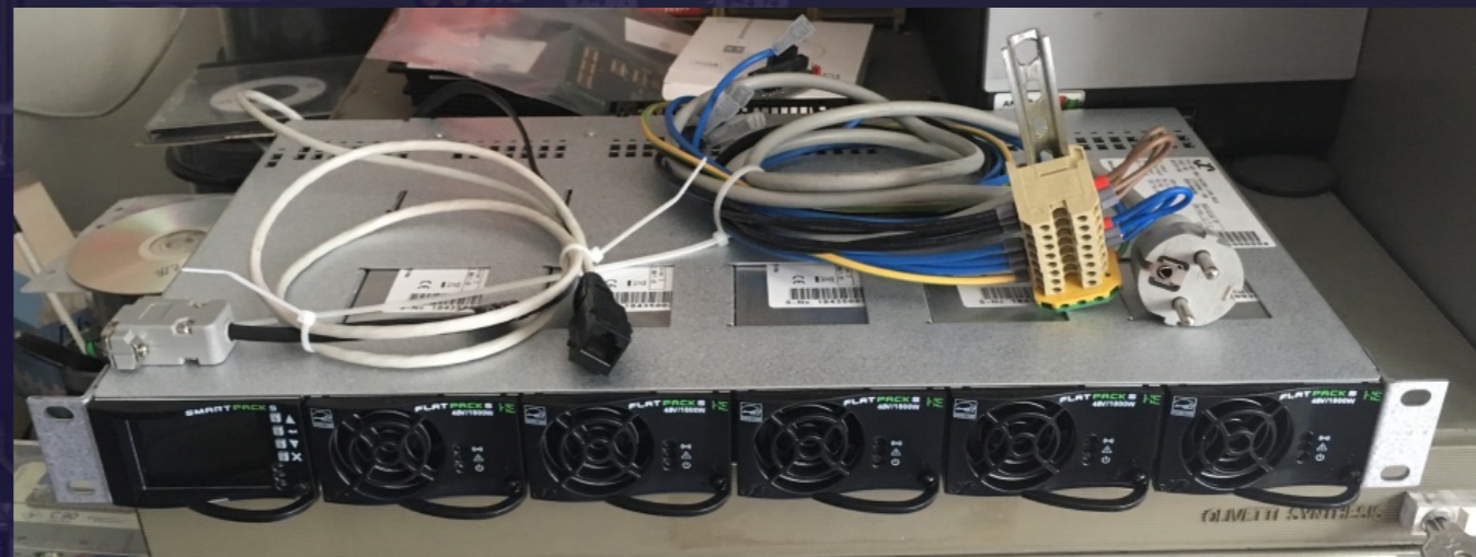
Power supply Eltek FlatpackS -48V 9kW 1U
