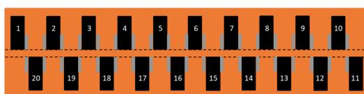
We developed an inverse analysis method to estimate the critical current density ( $J_c$ ) of each bulk from the measured field. After disassembly, sorting and reassembly, the magnetic field quality improves. The number here represents the order the  $J_c$  factors.
