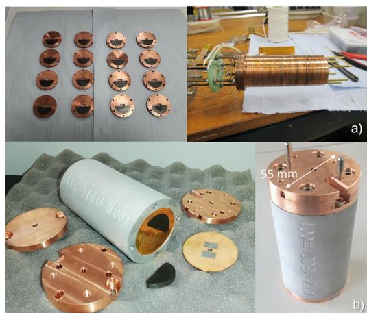
a) Cambridge GdBCO sample. b) ATZ YBCO + Cobalt-Iron poles, first industrial short sample. The HTS crystals are embedded (shrink-fit) into a copper matrix with micro-meter level accuracy, to be mechanically and thermally stabilised. An additional Aluminium shrinking cylinder is used to precisely assemble the undulator array.
