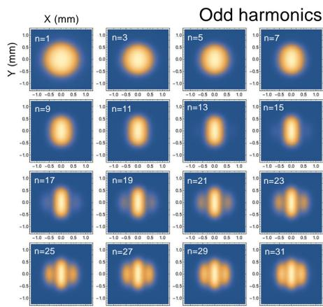
Calculations for the future I-TOMCAT beamline, dedicated to tomographic microscopy, flux at 30 m from the source to illuminate a sample of about 1 mm<sup>2</sup>
