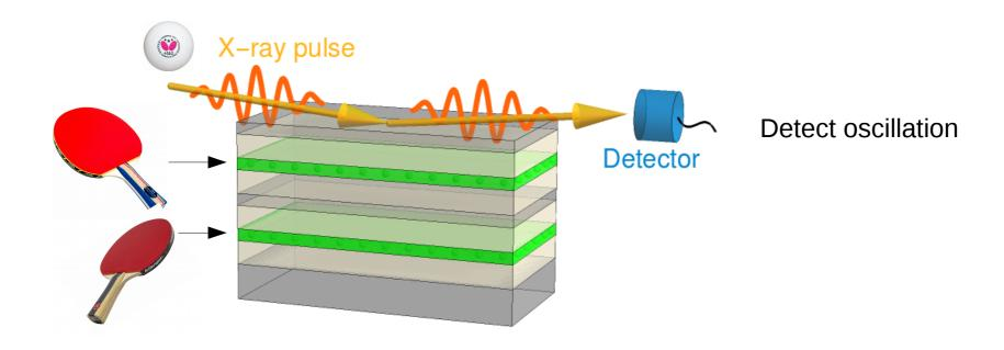
**Strong coupling:** the interaction between field and system is larger than the system decay rates.
