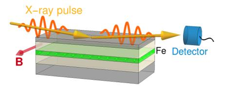
Successful quantum optics at single-photon level in thin-film cavitites – control of x-ray photons
