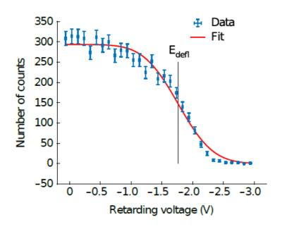
IC calculations to extract the energy value from the measured spectrum
