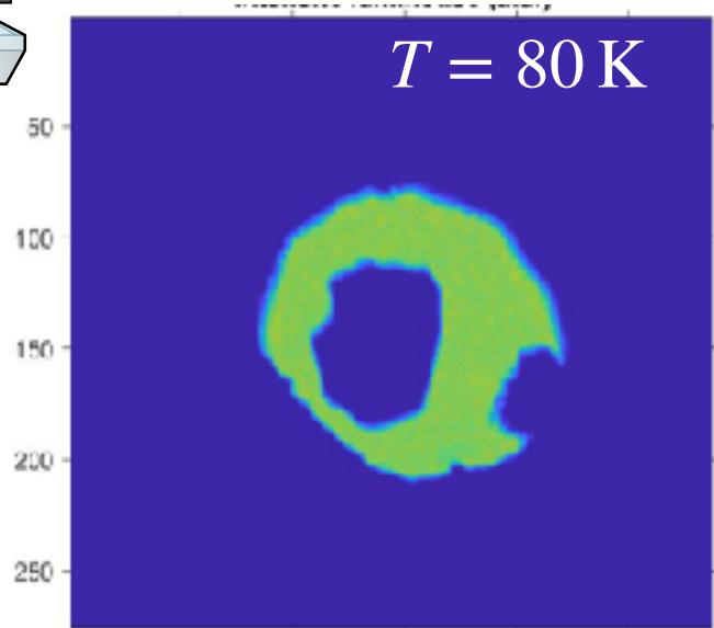
↑ NV luminescence detected by confocal microscopy
