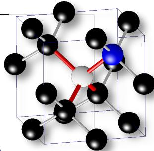
**NV color center in diamond:** electron spin that can be optically detected and manipulated by combining optical and microwave excitations
