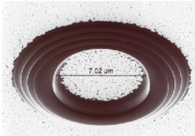
Diamond milling using Ga+ FIB
