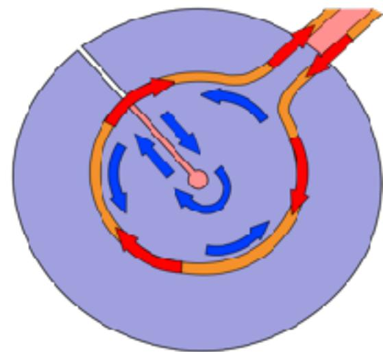
The slit cut in the metallic gasket avoids shielding but also behaves as a **focusing lens** for the microwave excitation
