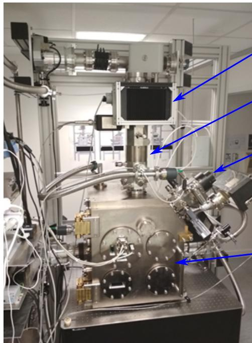
FIB with  $\text{N}_2^+$  or  $\text{Xe}^+$  beam
