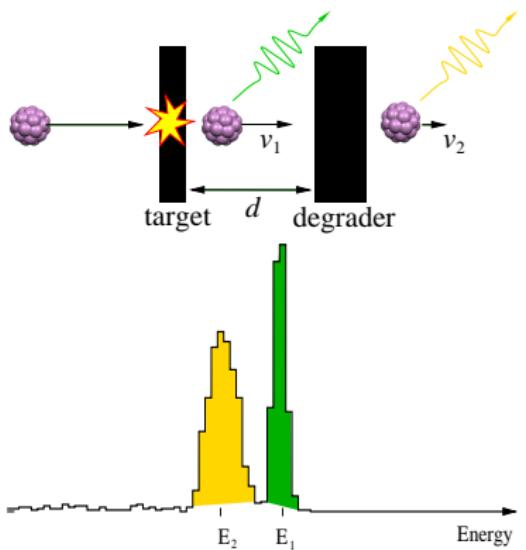
Doppler shift method for lifetime measurements
