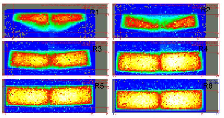
Detector scanned from side for 30s per position on a 1mm grid.
