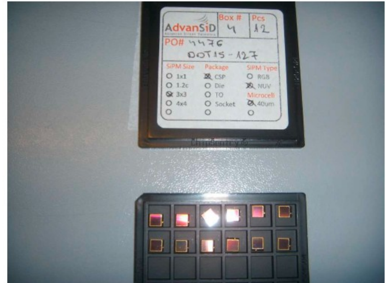
AdvanSiD NUV 3 \times 3 \text{ mm}^2 40 \mu\text{m} cells
