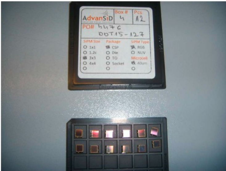
AdvanSiD RGB 3 \times 3 \text{ mm}^2 40 \mu\text{m} cells
