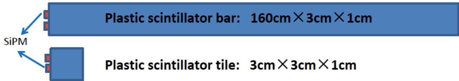
Two types of SiPM used as low and high channels to extend dynamic range.
