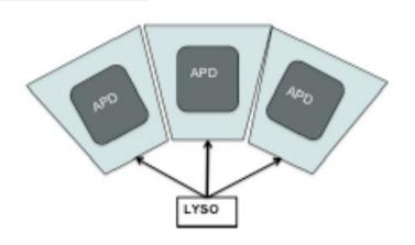
2 small barrels of 24 crystals each, with a length of 10-13 cm and transversal area from 1.5x1.5 cm<sup>2</sup> to 2x2 cm<sup>2</sup>
