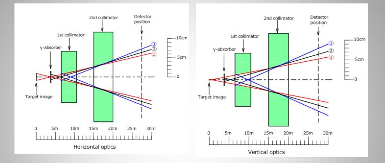
Rectangular shape to fit effective shape of target Two stages of long collimator made of iron To avoid multiple scattering inside collimator Bending Magnets to weep out charged particles Lead block to control photon flux
