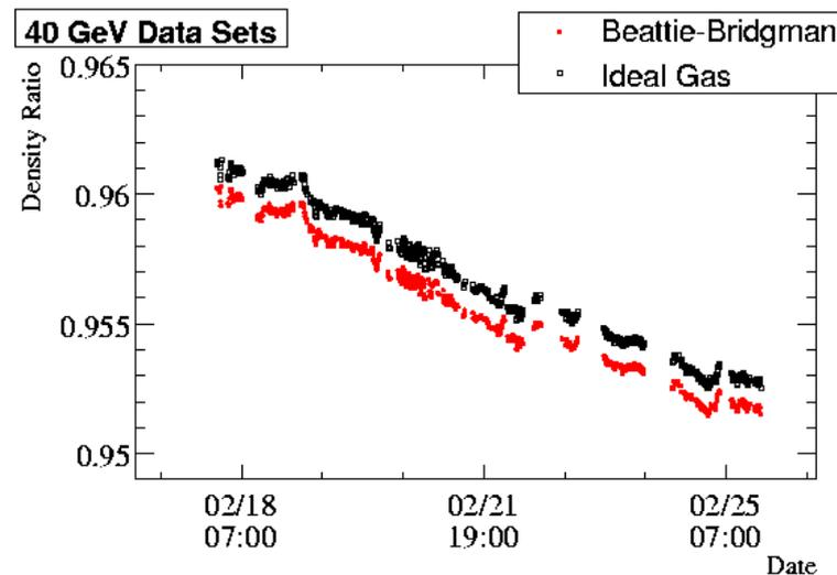
Vertical axis is current density divided by density at STP.
