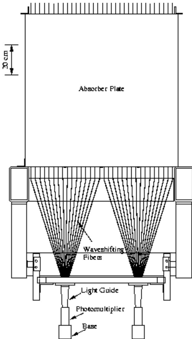
Measure forward going neutron production. Also functions as beam dump.
