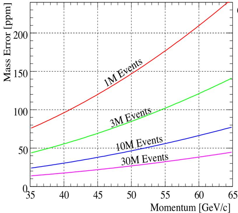
$\sigma_{m_K} \sim p^2 \rightarrow$  Need to run with momentum as low as possible. 40 GeV/c is still above proton threshold.
