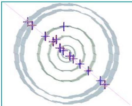
$\Delta_{xy}$  → distance between 2 half tracks in the xy plane at  $y=0$
