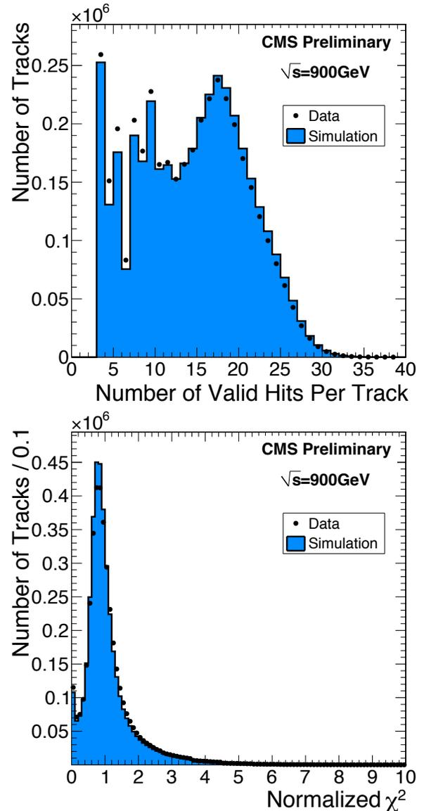
Figure 1. Representative low-level quality track distributions showing the number of tracker hits in a tracker track and the normalized  $\chi^2$  of the tracker track fits taken with 900 GeV c.m.s. energy.
