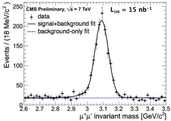
Figure 5. Uncorrected opposite-sign di-muon invariant mass distribution. Fit with a crystal ball signal shape on a flat background.
