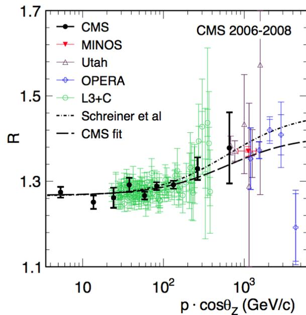
Figure 3. The CMS result for the muon charge asymmetry ratio as a function of the vertical component of the muon momentum, together with some previous measurements and a fit of the pion-kaon model to the CMS data.
