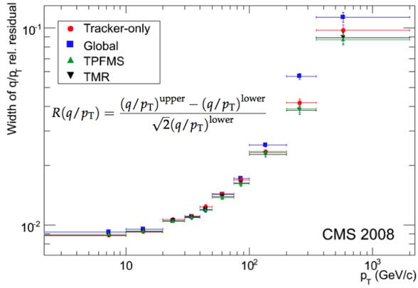
Figure 4. Widths of Gaussian fits to the distributions of the normalized residuals,  $P(q/p_T)$ , for various muon reconstruction algorithms, as a function of  $p_T$  of the reference track.
