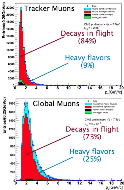
Figure 2. Comparisons between data and MC for the  $p_T$  distributions for global and tracker muons for  $0.2 \text{ nb}^{-1}$  integrated luminosity. Tracker muons are more efficient at low- $p_T$  but the sample has a higher fraction of decays-in-flight.
