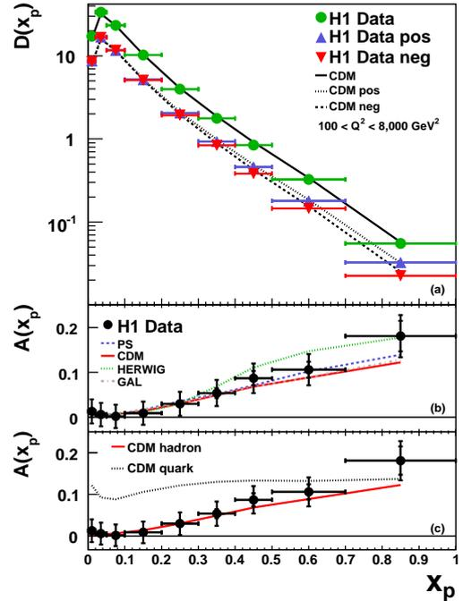
Figure 3. The measured normalised distributions of the scaled momenta for all charged particles and for positively (pos) and negatively (neg) charged particles (a), and the charge asymmetry as a function of  $x_p$  (b,c). The data are compared to predictions from different Monte Carlo models.
