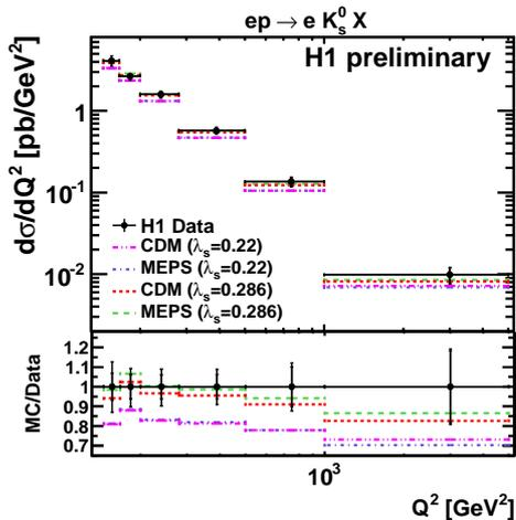
Figure 6. The differential production cross section for  $K_S^0$  mesons. On the bottom of the figure the "MC/Data" ratios are shown for different MC predictions. For comparison, the data points are put to one.
