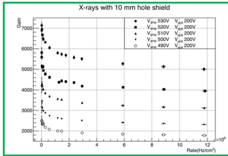
Gain reduction ~30% up to 12 MHz/cm<sup>2</sup> [CHARGING-UP + Ohmic Voltage Drop]
