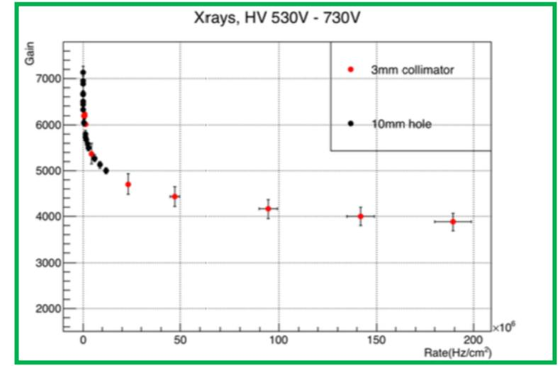
Gain drop increases as rate goes up. Still able to reach gain of  $4 \times 10^3$  at a rate of 150 MHz/cm<sup>2</sup> of 8 keV photons
