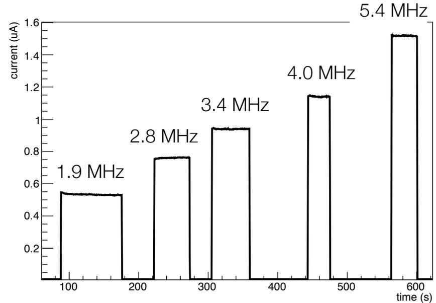
Current measurement Vs Time with X-Rays on/off and increasing rate (X-Ray current) at each step
