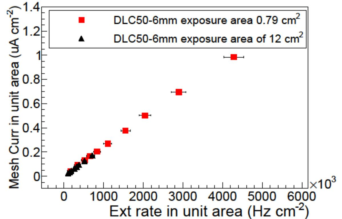
PAD-P: Response to illumination on 0.79 cm<sup>2</sup> and on 12 cm<sup>2</sup> does not show any significant difference up to the measured limit of ~8 MHz/cm<sup>2</sup> (total current was ~18 uA, close to the limit of the power supply)
