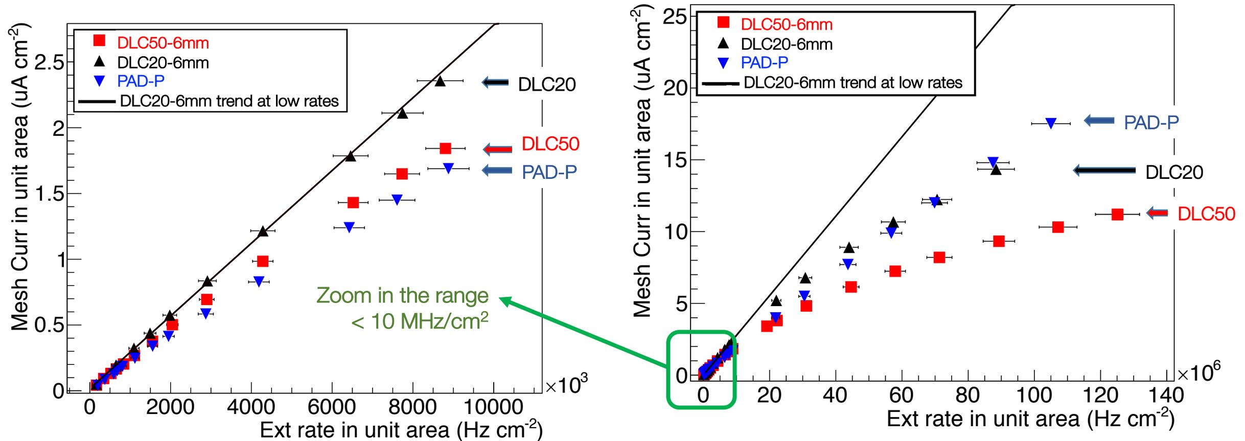
DLC20-6mm shows a significantly better behaviour than DLC50-6mm (LOWER RESISTIVITY)
