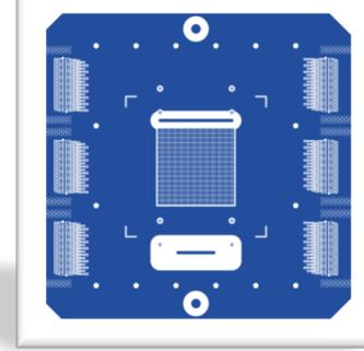
**GOAL:** Development of Resistive Micromegas detectors, aimed at operation under very high rates ( $\sim 10$  MHz/cm<sup>2</sup>)
