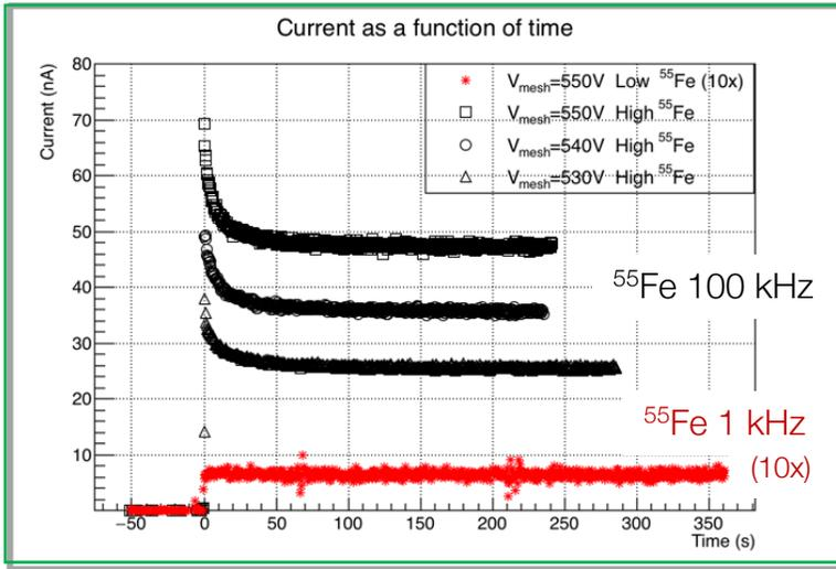
Reduction vs time of the detector current with High intensity  $^{55}\text{Fe}$  source [CHARGING-UP]
