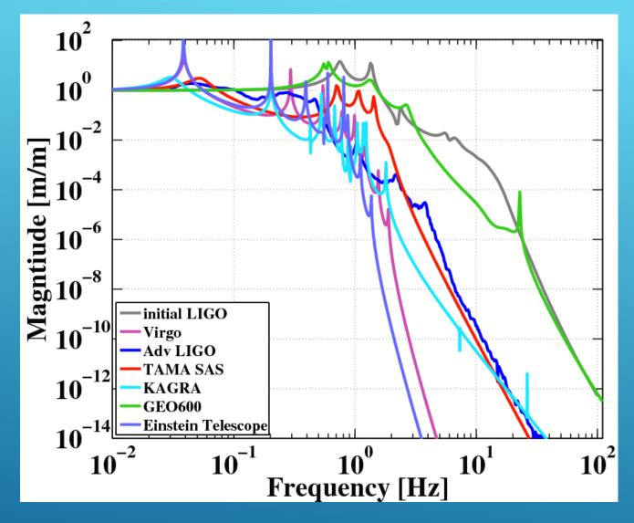
**Mechanical Transfer Function of different** vibration isolation systems
