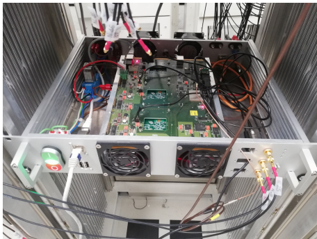
8 PMT connected to the 3 GCU | Trigger on threshold, BEC provides the OR of the 8 channels Data acquired and stored on 5 th of July (data taking 20 minutes)
