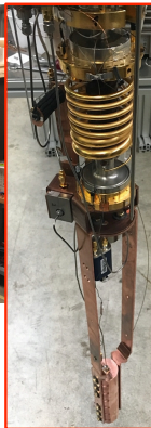
Dilution insert with rf electronics and cavity
