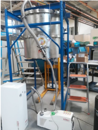
Leak test at room temperature
