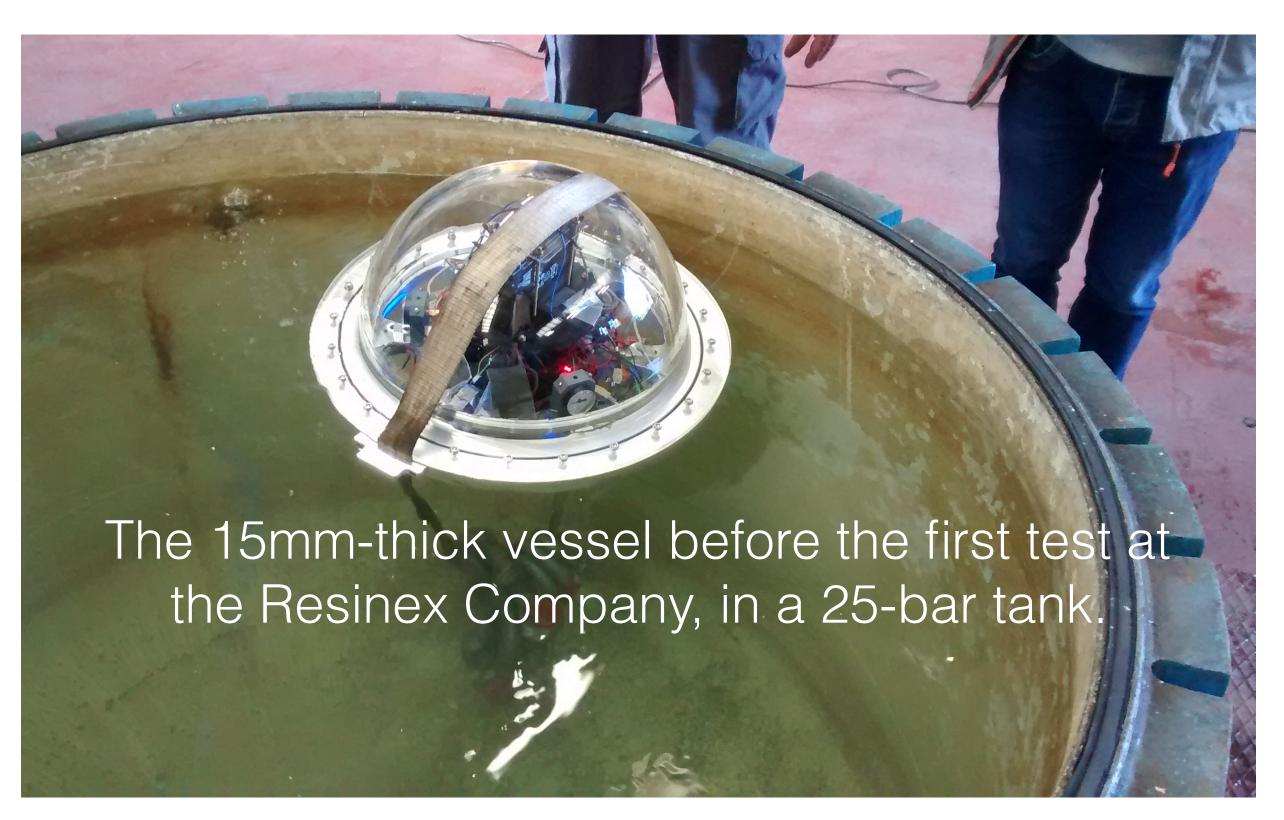
Our constrain was to resist up to 1.26 MPa and our vessel resisted to 18 bar (1.8 MPa).
