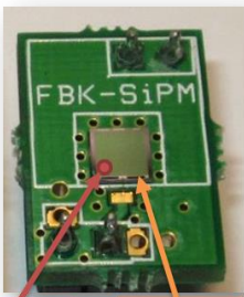
200µm SPOT 3x3mm² SiPM
