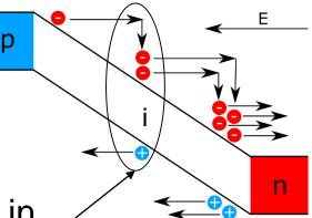
a free electron hits an electron in the valence band obtaining an additional free electron + a hole
