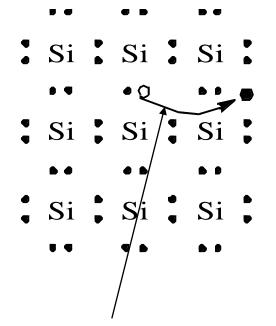
one **electron** can break the bond and become a **free carrier** (negative charge) the **hole** that is left can move too: free carrier with positive charge
