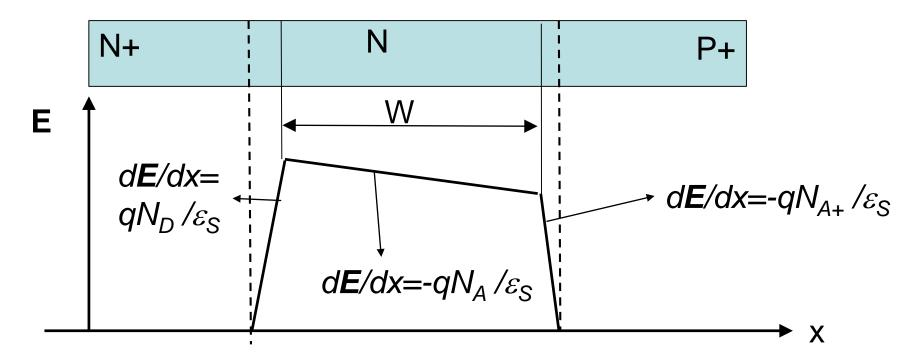
insertion of a low-doped region: trapezoidal electric field profile → same "area" with lower peak electric field
