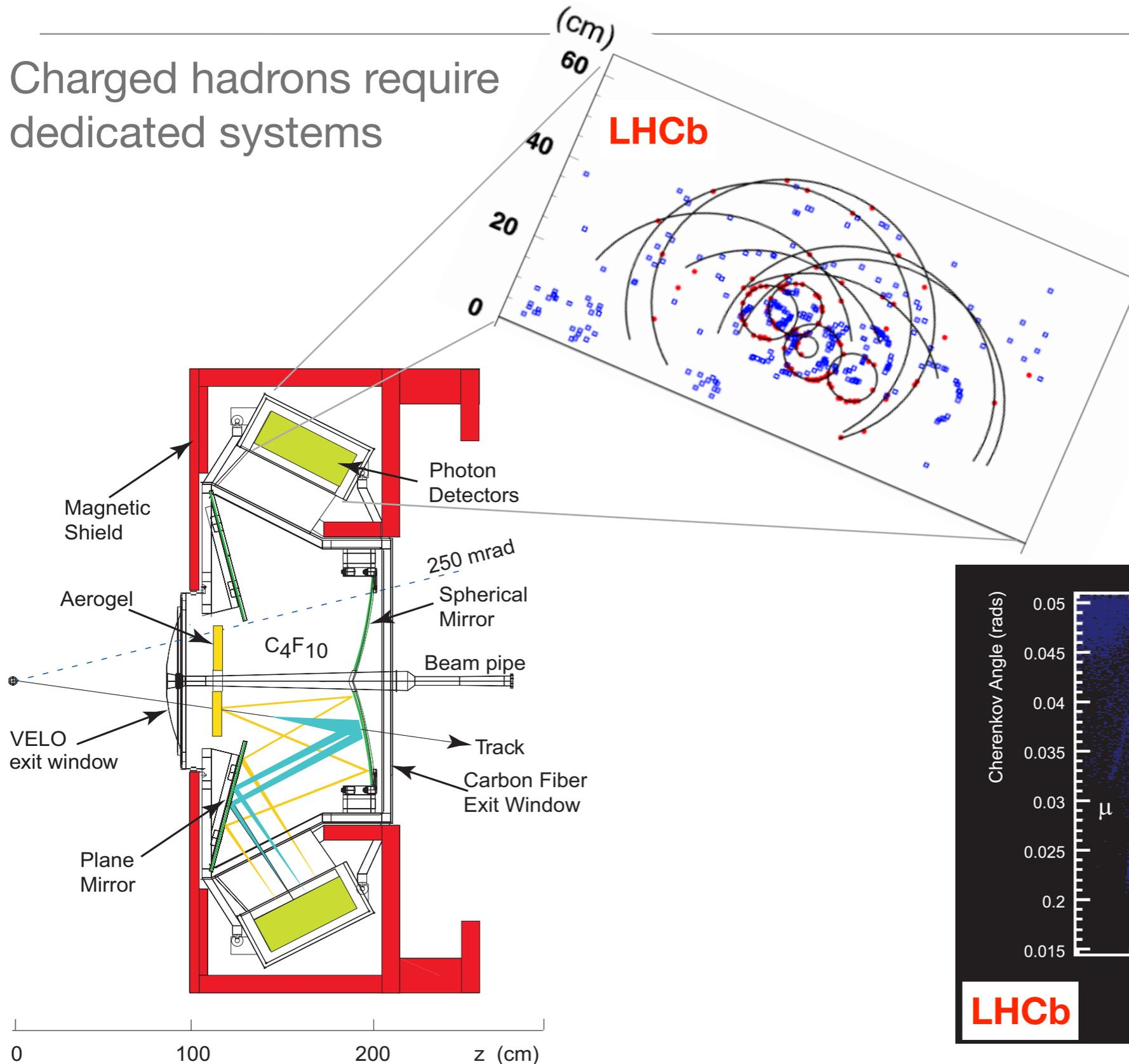
Systems based on Cherenkov radiation (BaBar, Belle, LHCb) offer best performance  $K/\pi$  separation  $> 5\sigma$  over a wide range in momentum
