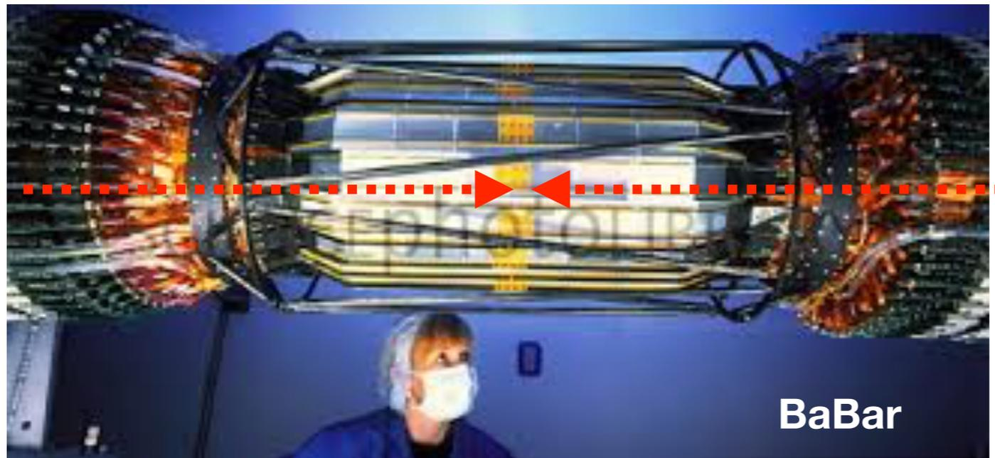
With  $c\tau \approx 0.5$  mm,  $B$  hadrons fly 0.5 to 50 mm. Measure the decay position by sampling precisely the trajectories of charged decay products close to the beam
