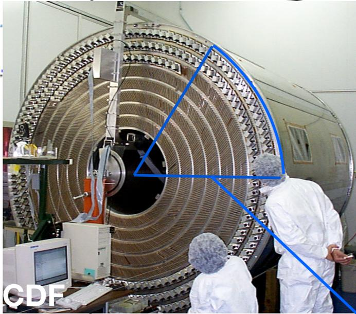
Measure accurately charged-particle momenta by sampling their trajectories curved by magnetic field along **large radii**.
