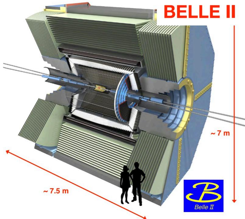
Classic: barrel-shaped solenoidal magnetic spectrometers
