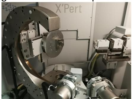
RCs are acquired along a direction, the angular shift corresponds to the tilt of crystal plane
