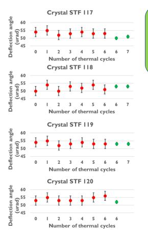
Although different expansion coefficient, crystal and holder maintain perfect mounting within µm
