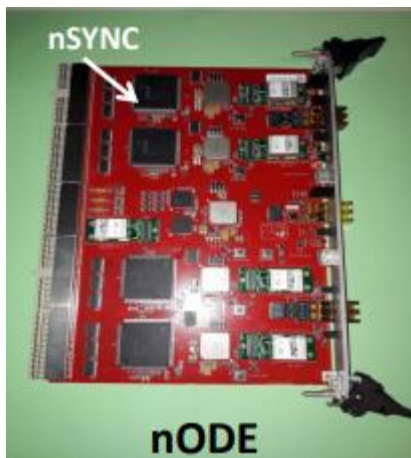
Data readout at 40MHz: nODE boards, equipped with nSYNC ASIC (4 per Board)
