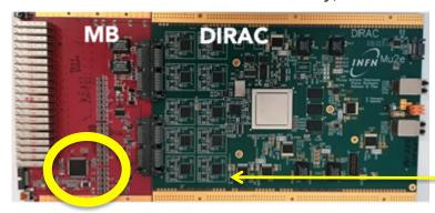
Few SEU observed up to 1.5E<sup>10</sup> p/cm<sup>2</sup> due to Ethernet connection. Repeat with final MB
