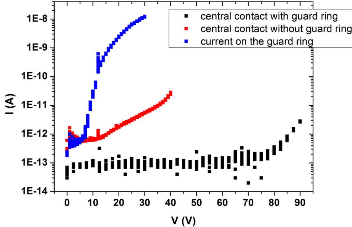
Central contact low level of leakage current,  $<1\text{pA}$  @ 80V
