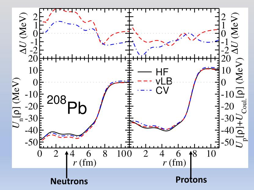
Lower panel: **vLB** and **CV** potentials from <sup>208</sup>Pb density corresponding to SkX **HF** potential.
