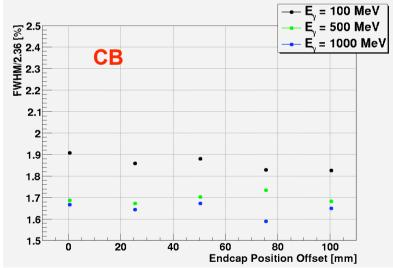
Scan Energy resolution as a fuction of Forward Endcap position with respect to the Barrel
