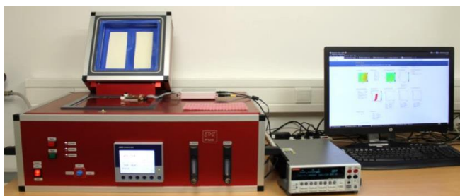
CMS pixel detector module testing setup & DAQ
