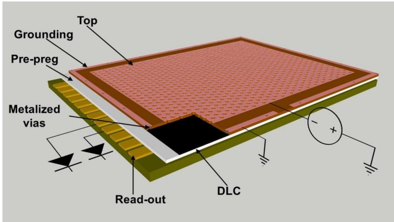
**Single Resistive Layer (SRL):** a simple 2-D current evacuation scheme based on a **single resistive layer** with a **conductive grounding** all around the **perimeter** of the active area.
