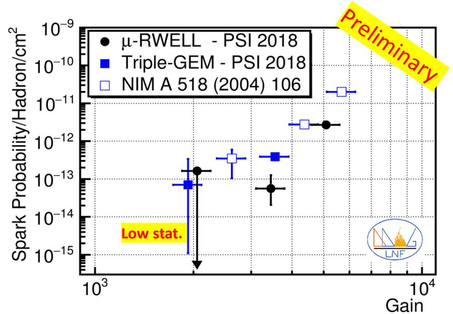
The discharge probability for  $\mu$ -RWELL comes out to be slightly lower than the one measured for GEM.
