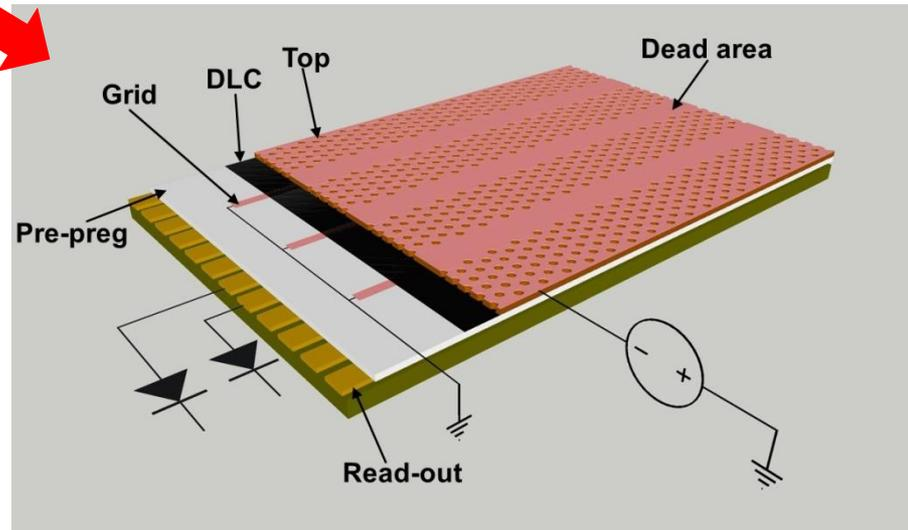
Single resistive layer with dense grid grounding
