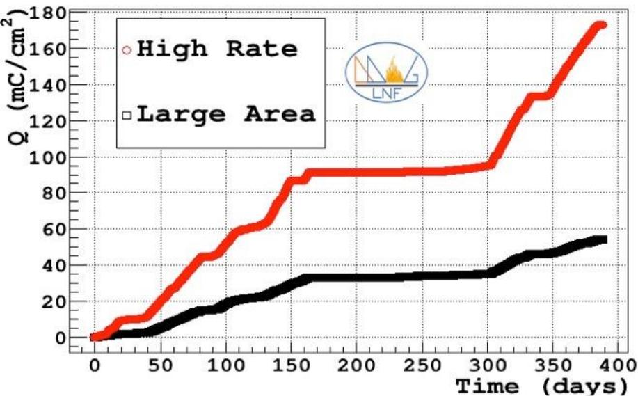
TB PSI – beam spot 9 cm<sup>2</sup> – flux ~ 10 MHz/cm<sup>2</sup>
