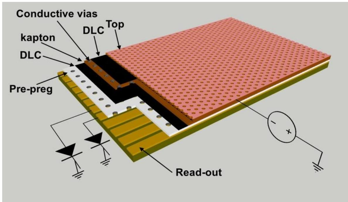
**Double Resistive Layer (DRL):** 3-D current evacuation scheme based on two stacked resistive layers connected through a matrix of conductive vias and grounded through a further matrix of vias to the underlying readout electrodes. The pitch of the vias can be done with a density less than  $1/\text{cm}^2$ .
