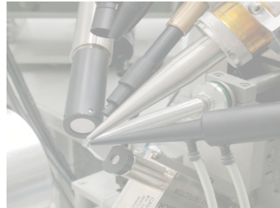
External beam with scanning microprobe with detectors for PIXE, PIGE and RBS/EBS analysis
