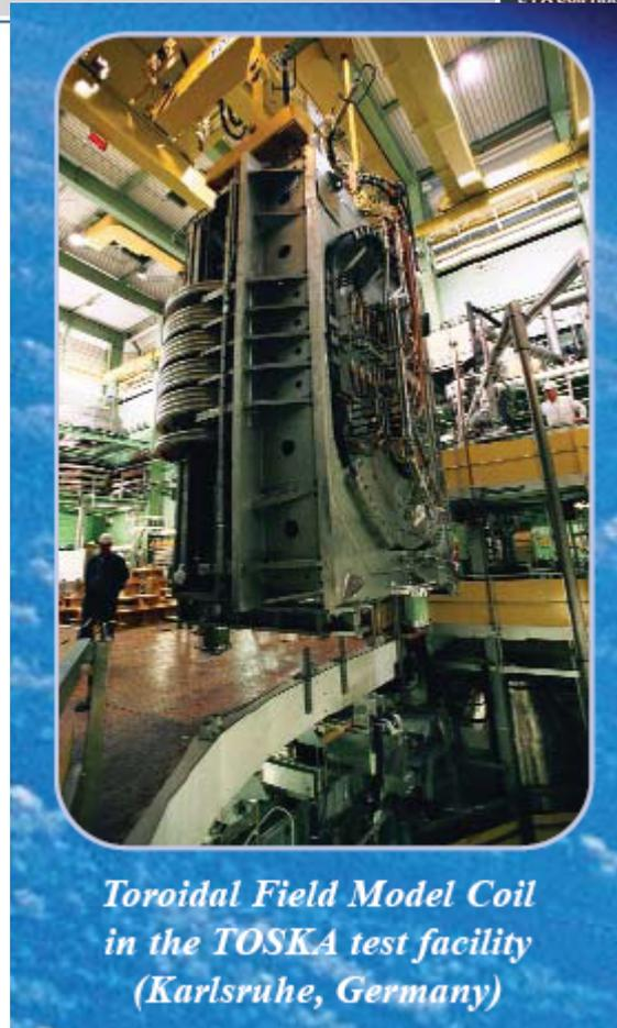
*Toroidal Field Model Coil
