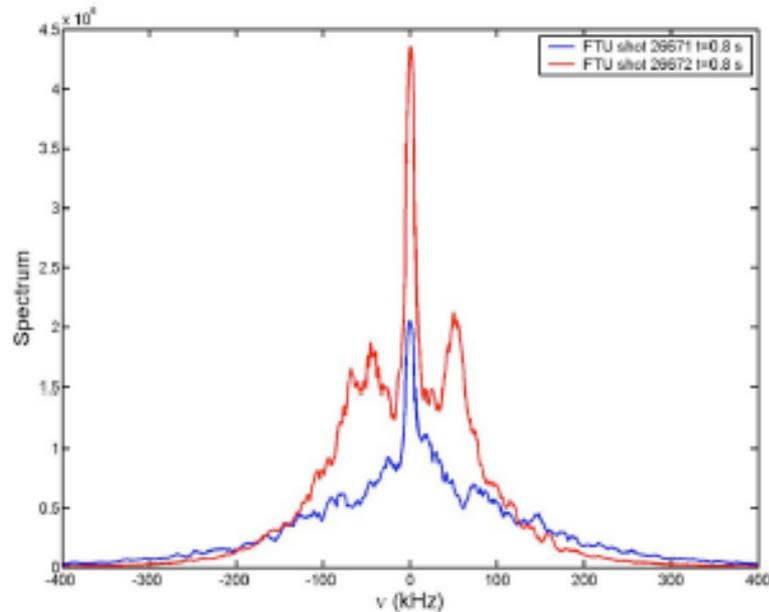
Fig. 4 – Fluctuation power spectra for two discharges with ITB (#26671, blue) and without (#26672, red);  $n_e \approx 0.9 \cdot 10^{20} \text{ m}^{-3}$  for both
