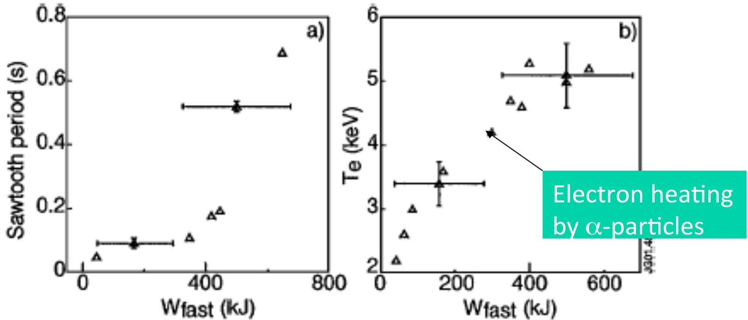
FIG. 4. Sawtooth period (a) and ECE  $T_e(r/a \approx 0.25)$  (b) as functions of the fast ion energy  $W_{fast} = 2(W_{DIA} - W_{th})/3$  for discharges with  $\omega \approx 3\omega_c(^4\text{He})$  and 1.5 MW of 120 keV beams. Here  $W_{th}$  is the thermal stored plasma energy deduced from measured plasma densities and temperatures.
