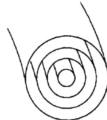
Fig. 3.2.1 Magnetic flux surfaces forming a set of nested toroids.
