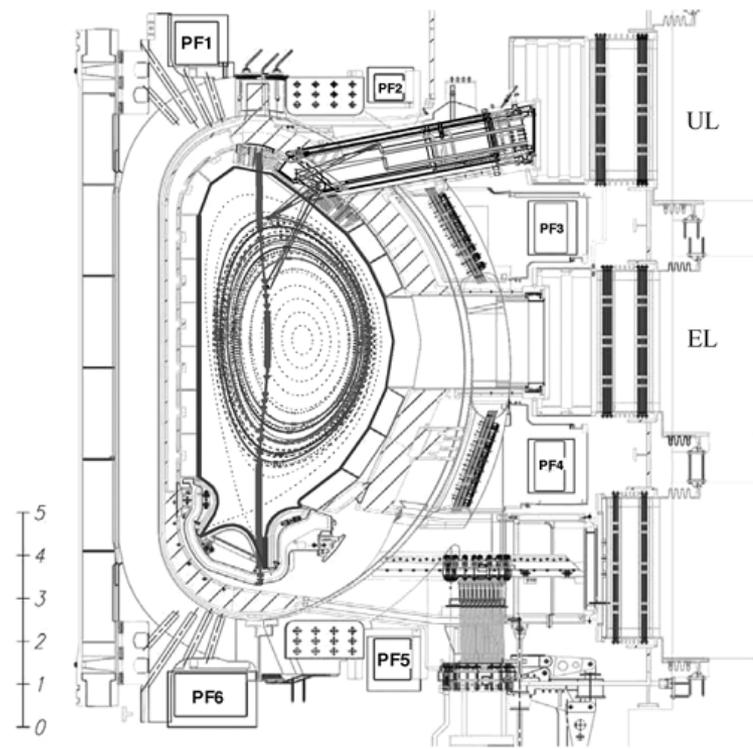
**Figure 1.** The cross section of ITER with the location of the EL and UL ports identified. A simplified UL is placed in the upper port with the beams aimed at the innermost and outermost expected locations of the NTMs.
