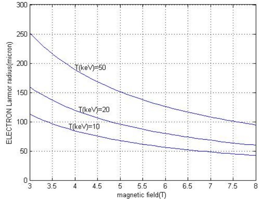
$$\rho_e = \frac{v_{\perp e}}{B} = 1.07 \cdot 10^{-4} (T_{e\text{keV}}^{1/2} / B) \text{ m}$$
