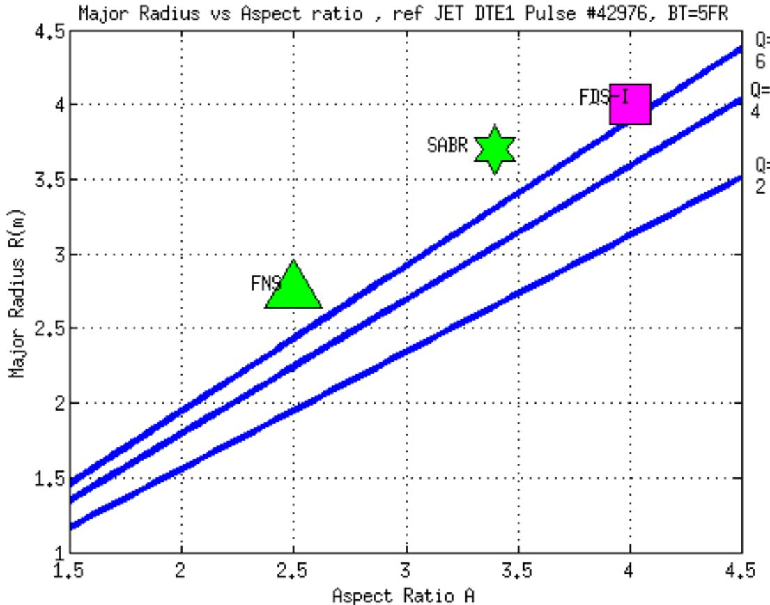
The blue lines are calculated using the  $S_{FR} = R B^{4/3} A^{-1} * Q_0^{1/2}$  Scaling law, fixing the magnetic field  $B = 5T$ , and taking as reference the plasma parameters of JET DTE1 Pulse #42976.
