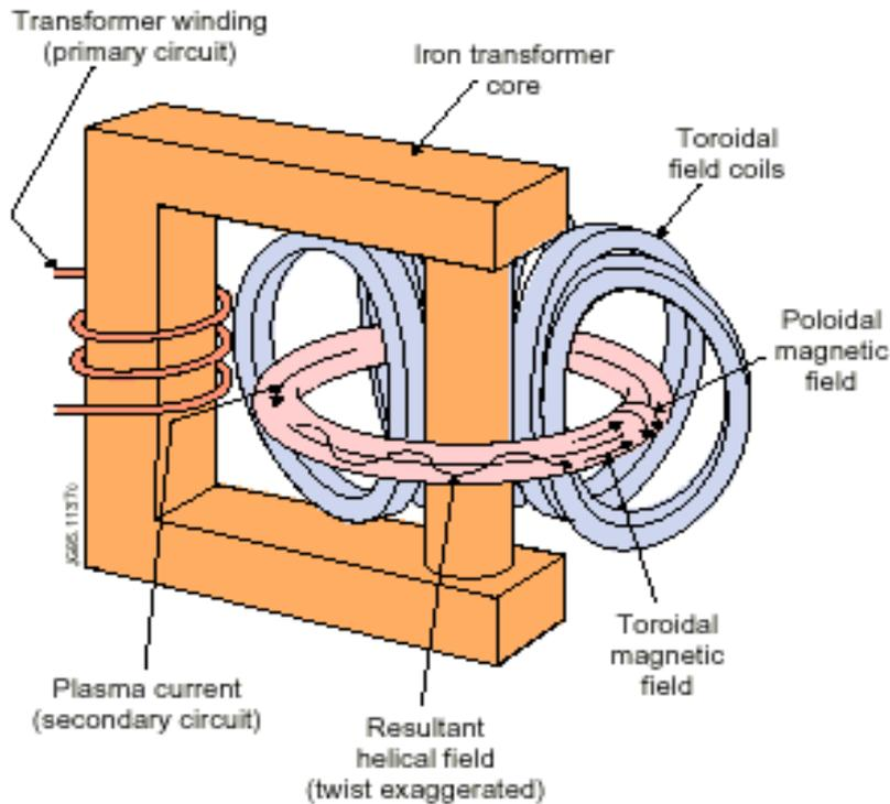
In a plasma contained in a toroidal device with axial magnetic field a current is induced by a transformer
