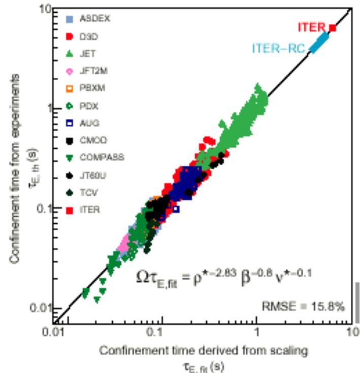
Experimental Scaling law confinement time for magnetic confinement tokamak devices (H-mode)
