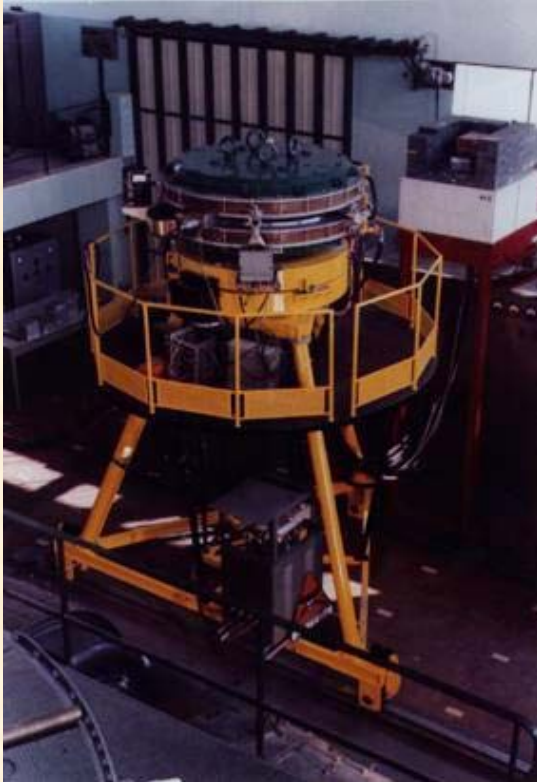
AdA, the first electron-positron collider: 2 m diameter, 250 MeV.
