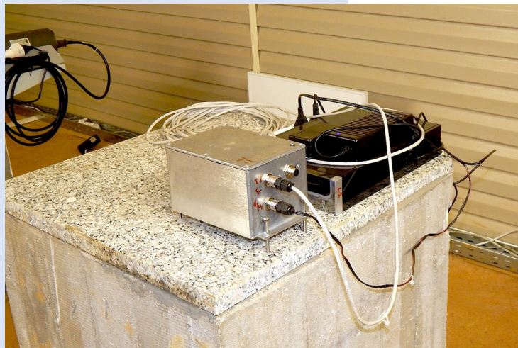
Seismometer of Warsaw University: three geophones in the metal housing
