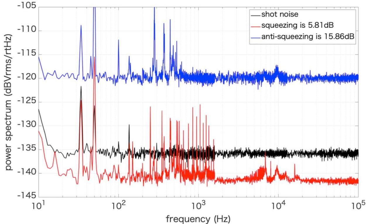
Typical squeezing spectrum:
