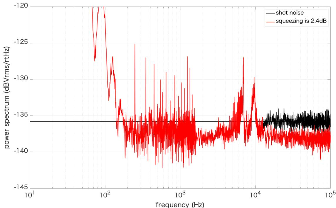
Squeezing measurement with unlocked FC:
