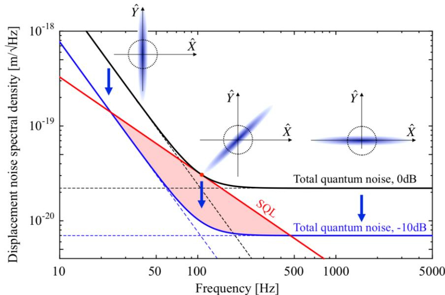
To achieve broadband quantum noise reduction, injection of frequency dependent squeezed vacuum (which is phase squeezed at high frequency and amplitude squeezed at low frequency) is required
