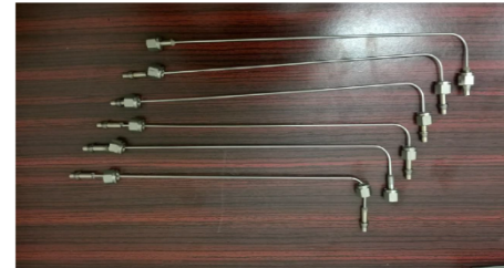
PIPE -CUSTOM MADE- AISI 316L ID 2.0 mm, OD 2.5 mm SWAGelok COMPRESSION FITTINGS GLUED WITH EPOXY 2011 TESTED WITH CO2 PRESSURIZATION AT ~ 60 bar + HELIUM LEAK-CHECK IN MILANO
