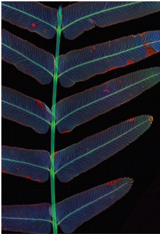
Figure 2: Maia image (Ca As K as RGB) of a live Pteris vittata frond from a scan measuring 58 \times 85 \text{ mm}^2 , 2901 \times 4251 pixels (12 M pixel each 2 ms, 20 \mu\text{m} ), acquired at 15.8 keV incident energy on the XFM beamline, AS.
