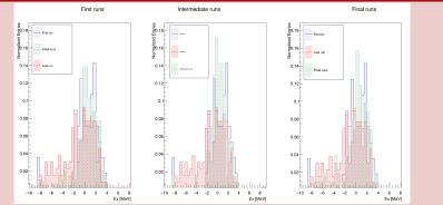
breaking up Ex over various runs show that a time-dependent energy correction must be included
