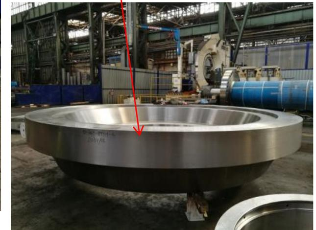
Cradles 2 main parts are in progress: 1.47x4.15x7.68, m; 34 tons in total
