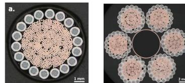
A demonstrator (2 x 60-m long, 18 kA cables) tested in Dec. 2018, exceeding requirements -  $T_{CS}$  at 18 kA of 31.3 K
