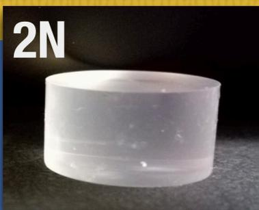
The 2N sample is less transparent than, for example the 2B, however it doesn't need any dopant to reach important light output values. A concentration study has been then performed.
