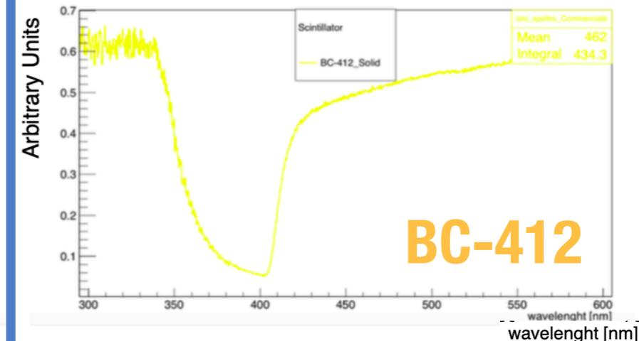
The new plastic scintillator samples have been characterised in terms of transmittance and emission with photoluminescence spectroscopy measurements.
