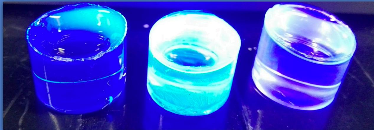
The possibility of developing plastic scintillators with our molecules was demonstrated using a system of a polyvinyl-toluene (PVT) polymer matrix loaded with various concentrations of scintillating compounds.
