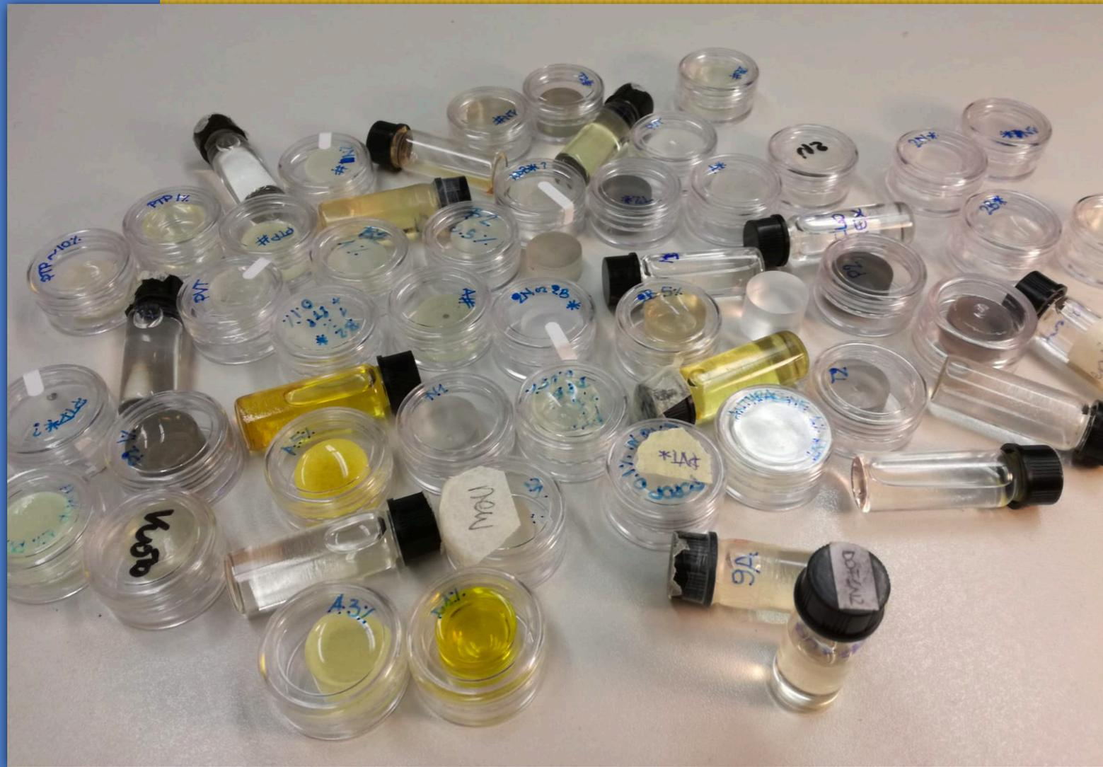
Both liquid and solid samples have been tested with cosmic rays (mip) and the light output produced by ionisation in the scintillators has been collected with a commercial PMT.
