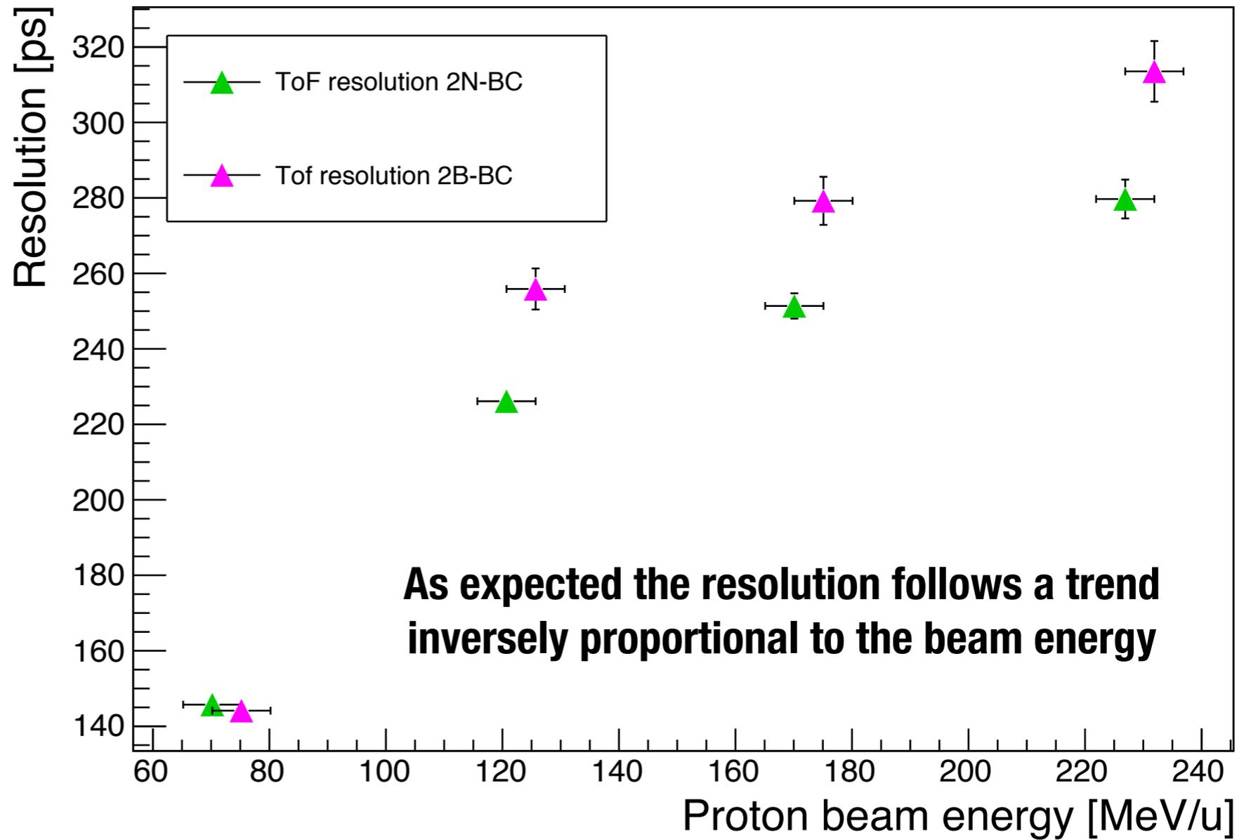
Measurement of Time Resolution in proton Time of Flight (ToF)
