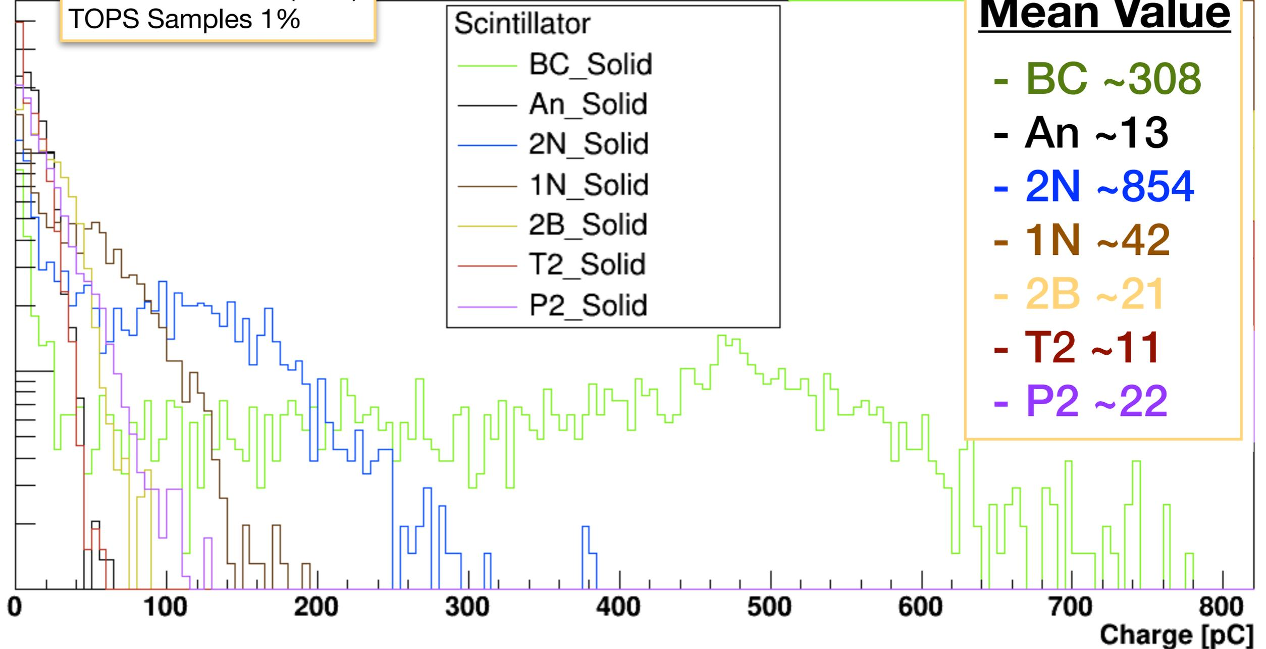
As expected the commercial scintillator shows much better performances, however it has to be stressed that the TOPS scintillators are not jet optimised in terms of concentration and transparency.
