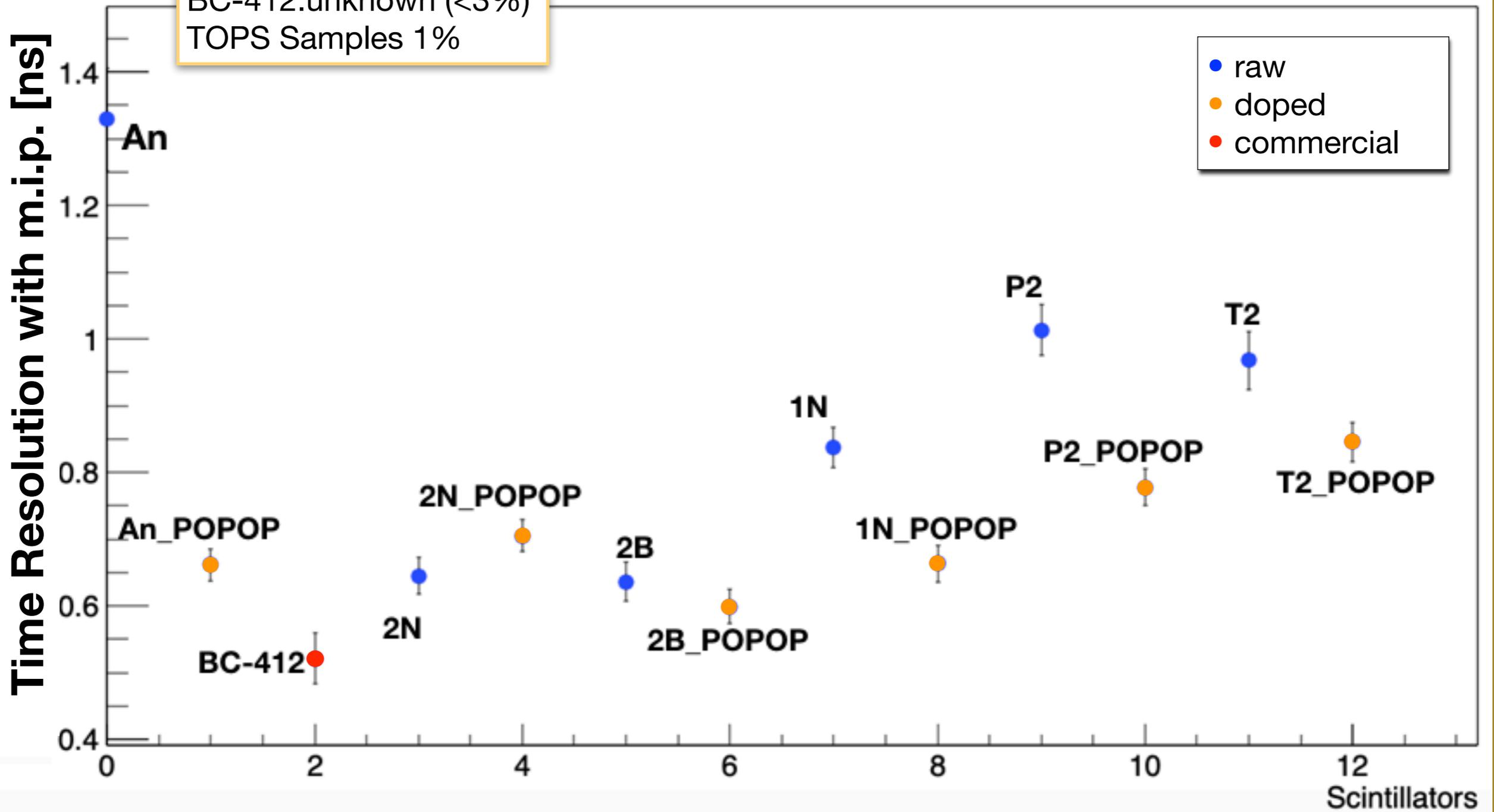
A very promising time resolution of  $\sim 600$ ps for 2N e 2B (BC-412 500ps) is obtained with this readout and setup. A preliminary time characterisation has been performed for those two samples.
