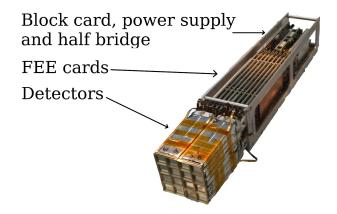
**16 telescopes**, together with **front-end electronics**, form a **block** operating in **vacuum**.
